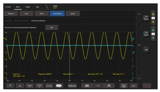
Tap **OK** on the pop-up message box to start calibration. The LED on the EM101N starts flashing and the prompt message "Calibrating, please wait" will appear on the upper left corner of the screen.
