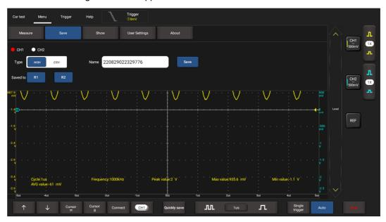
Select the desired measurement channel, select file type (.WAV or .CSV), tap the default file name to change the file name and select save. Alternatively, the user can save the waveform files to the designated folder (R1, R2). If the files are saved under this folder, the user can recall the saved files for reference and play back through REF channel.
