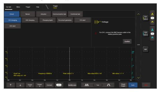
Tap to select the desired automotive part, the system will automatically configure the option to the preset parameters. The user does not need to make any settings. Just follow the on-screen instructions to make connections and proceed.
