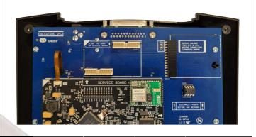
INSERT SERVICE BOARD CAN-FD INTO THE CONNECTOR AS IN THE PHOTO BELOW,
